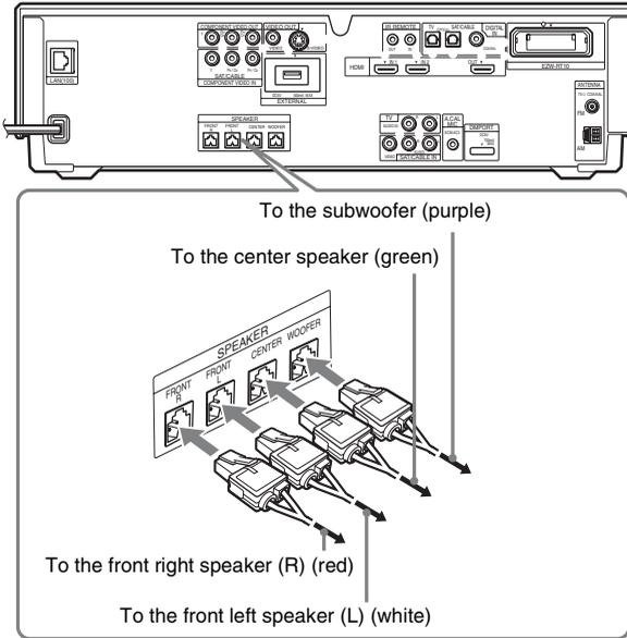
When connecting the speaker cords to the subwoofer, use the speaker cords (purple). Be sure to match the speaker cords to the appropriate terminals on the speakers: the speaker cord with the color tube to  $\oplus$ , and the speaker cord without the color tube to  $\ominus$ . Do not catch the speaker cord insulation in the speaker terminals.
