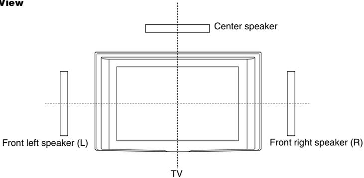
Position the front speakers so that their centers align with the TV. Position the center speaker so that the center of the speaker and the TV are aligned.
