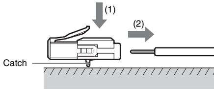
When attaching the speaker cords to the connector, be sure to match the polarity of the speaker cords and the connector.
