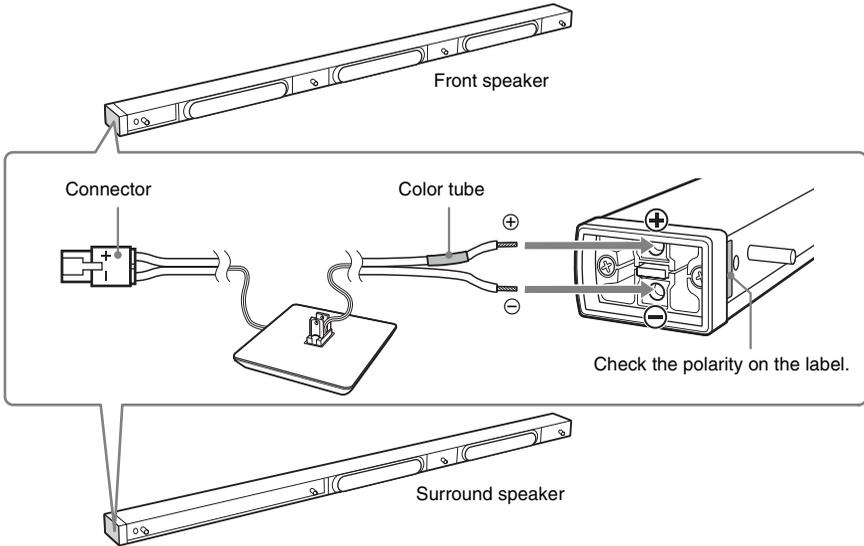
Insert the speaker cords into the speaker terminal of the speaker as far as they will go. Ensure that the cords are secure by gently pulling on them one at a time.
