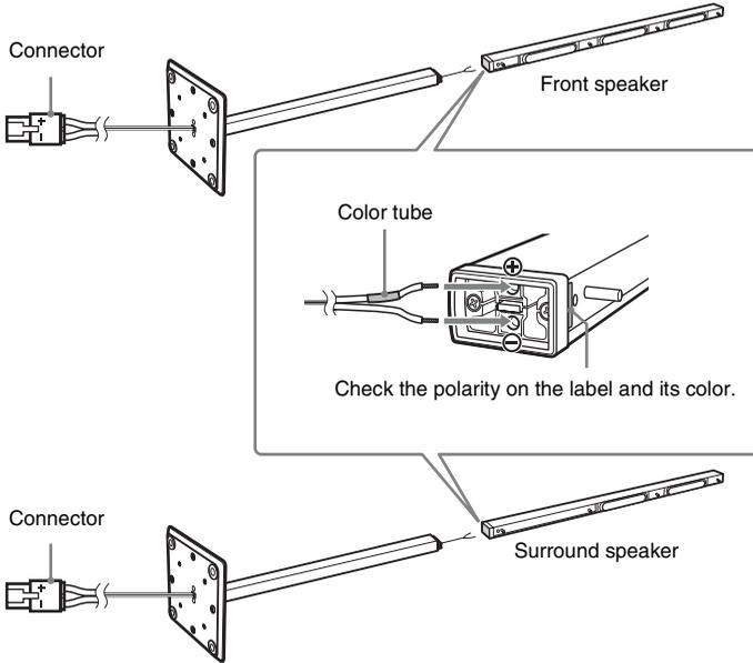
Insert the speaker cords into the speaker terminal of the speaker as far as they will go. Ensure that the cords are secure by gently pulling on them one at a time.
