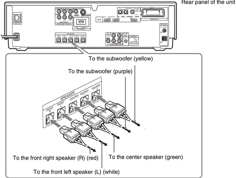
The speaker cords (yellow and purple) are connected to the subwoofer beforehand as follows. When re-connecting, be sure to match the speaker cords to the appropriate terminals on the speakers: the speaker cord with the color tube to  $\oplus$ , and the speaker cord without the color tube to  $\ominus$ . Do not catch the speaker cord insulation in the speaker terminals.
